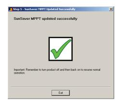
**G)** Reboot the controller by disconnecting the battery/supply POSITIVE from the controller, waiting 10 seconds, and then re-connecting the wire.
