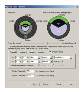
**F)** The slider bar can be dragged from left (winter) to right (summer) in order to give a visual representation as to how the lighting/load behavior will change with the seasons. *Note: The position of this bar does not affect the load control configuration, it is simply a visualization tool.*
