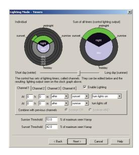
**C)** Click on the Channel 2 tab to make Channel 2 active. Configure the action drop down box to read **Do Nothing**. This will cause Channel 2 in the left graph to go dark, indicating Channel 2 is no longer contributing to the lighting/load control and has been disabled. (This may or may not cause a change to the right graph.)
