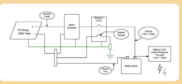
One of the main issues with other ground fault detection/interruption (GFDI) products is that these all break the bond to the grounded conductor. When this occurs, not only is the earth bond compromised but the battery and DC loads can also be left ungrounded and floating. For a negatively grounded system this means that the negative side of the battery and loads can float to negative Voc in relation to ground and the positive side can float to (negative Voc + Vbat).
