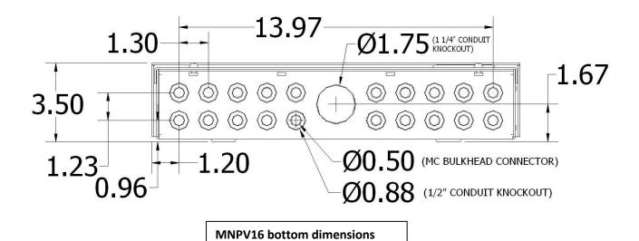
PV input knockouts for these combiners are a dual concentric knockout that can accept bulkhead mount MC cable connectors. Configuring these enclosures with the bulkhead mount connectors in advance can save time in the field. Several brands will fit the ½" diameter knockouts.
