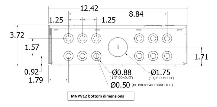
Two 7/8" knockouts (1/2" conduit openings) are located on the sides of the MNPV12. These are primarily intended for lightning arrestors. One 1 ¼" conduit knockout is located on the back mounting surface.
