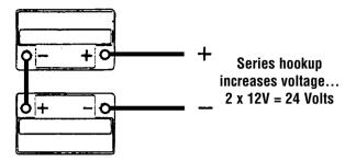
During recharge, each battery receives the same amount of current; e.g. if the charger is putting out 10 amps, both batteries are getting 10 amps.
