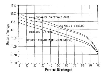
CHART E Gel Battery Capacity Voltage vs. Percent Discharged
