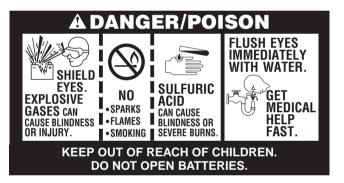
Because SVR batteries normally emit very little to no hydrogen gas, they are safe near sensitive electronic equipment. They do not cause corrosion of surrounding metals. No hydrogen gas means no dangerous explosions... UNLESS SEVERELY OVERCHARGED!
