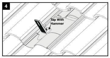
Place L-Foot over top of dimple and tap with hammer to punch the threaded posted through the flashing. Ensure punched pieces of flashing are cleared away.
