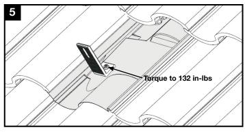
Form flashing as needed to sit flush with surrounding tiles. Position L-Foot in desired orientation and torque hardware to 132 in-lbs (11 ft-lbs).
