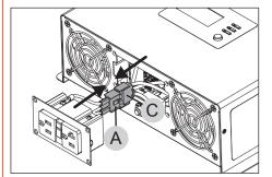
Attach the two connectors together  $A \rightarrow \leftarrow C$ .
