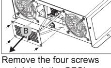
and detach the GFCI cover plate B from the inverter unit.
