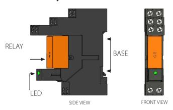
The FLEXware Relay Assembly will activate a two-wire start generator when wired to the AUX output of either an OutBack FX Inverter/Charger or an OutBack Charge Controller. The assembly consists of an LED module and a relay inserted (in one orientation) into a base. The base is mounted onto the DIN rail of any OutBack AC industrial control panel.
